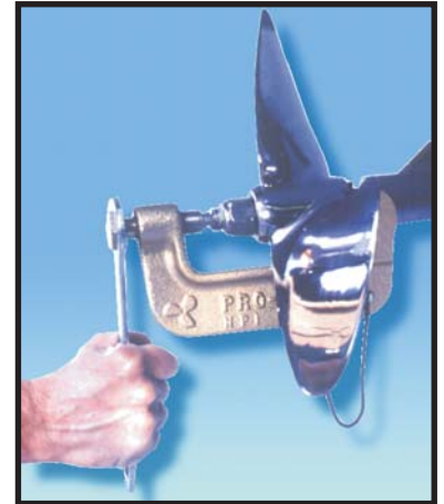
#102 In use on a 3 blade propeller with a 1" propeller shaft.
